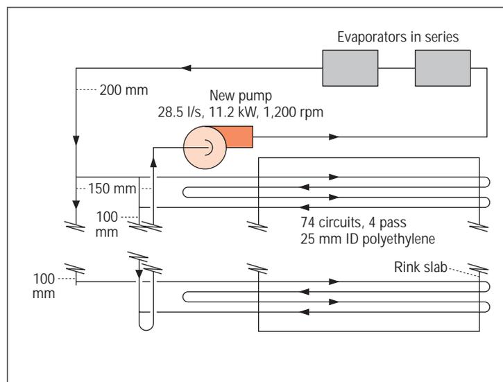
Figure 2: Schematic of four-pass system with evaporators in series.
