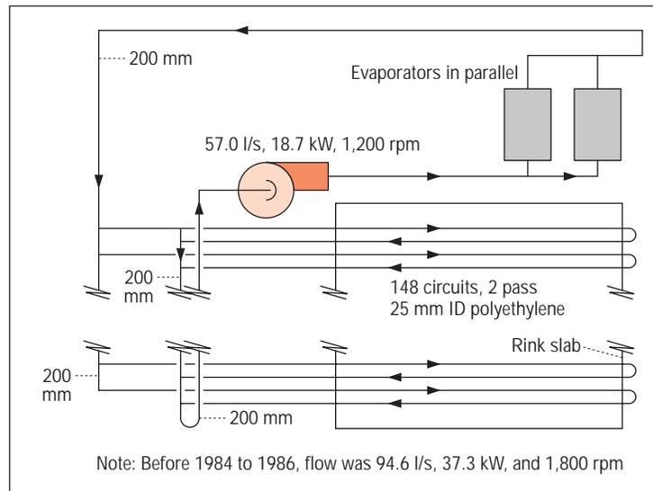
Figure 1: Schematic of two-pass system with evaporators in parallel.
