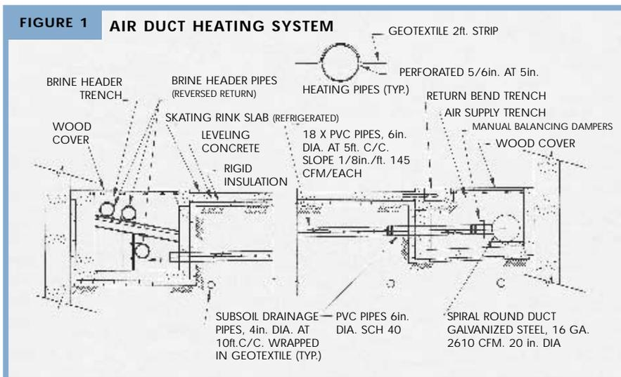
**FIGURE 2 SUBFLOOR HEATING/VENTILATING SYSTEM**
