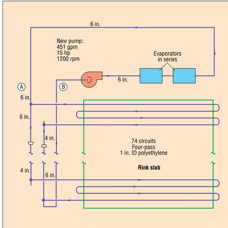
2 Schematic of four-pass system with evaporators in series (not to scale).
