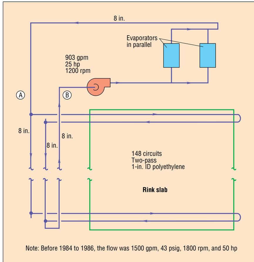
1 Schematic of two-pass system with evaporators in parallel (not to scale).
